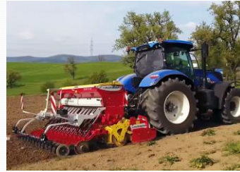
Pöttinger Agritechnica2017 SILVER measures the soil surface roughness using live images from a stereo camera mounted between the power harrow and the seed drill by ISOBUS III
